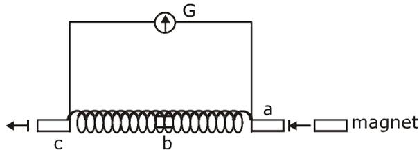
Three positions shown describe: (a) the magnet's entry (b) magnet is completely inside and (c) magnet's exit.
